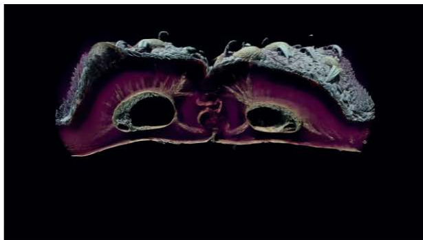
图1.铁铤甲虫鞘翅连接电子显微结构：资料来源Rivera, J., Hosseini, M.S., Restrepo, D. et al. Toughening mechanisms of the elytra of the diabolical ironclad beetle. Nature 586, 543 - 548 (2020).
