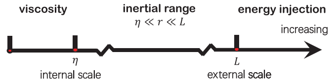
FIG. 5. Superimposed on the mean motion are turbulent pulsations of various length scales. It also shows Richardson’s idea of the existence in the turbulent flow of vortices on all possible scales between the external scale ( L ) (the Taylor’s Lagrangian integral scale) and the internal scale ( \eta ) (the Kolmogorov local scale of turbulence). Three regions: a region dominated by viscosity at the very smallest scales; an intermediate inertial range characterized by zero dissipation; and a region of energy injection (or energy-containing) at the largest scales.
